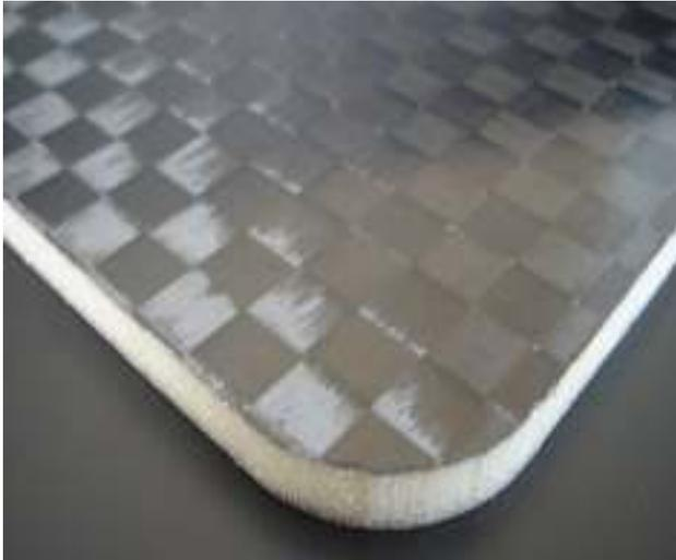
Fig. 6 Sandwich Composite Cut Out [9].
