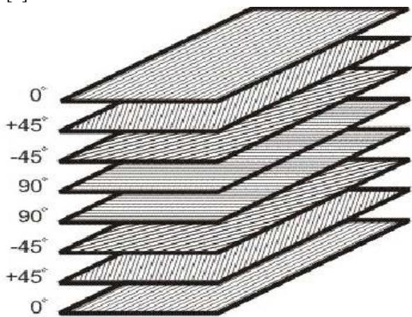
Fig. 3 Layering of Composite Materials at different angles [7].
