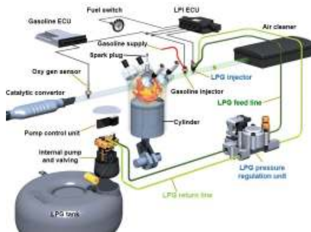
Fig. 12 LPG liquid phase injection system [8].
