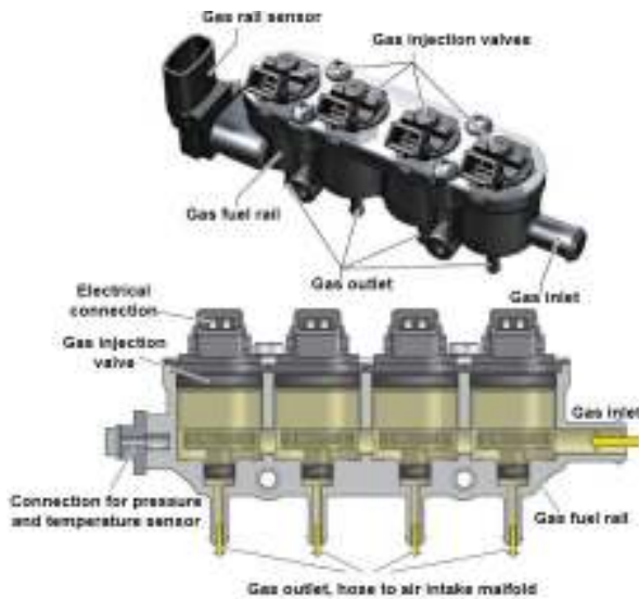
Fig. 10 LPG gas fuel rail, according to [7].
