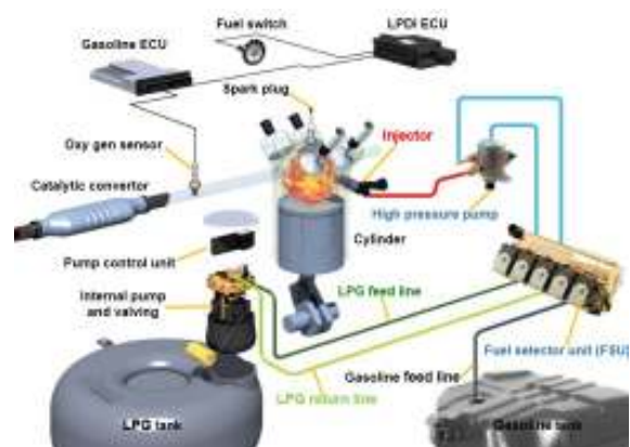
Fig. 13 LPG liquid phase direct injection system [9].
