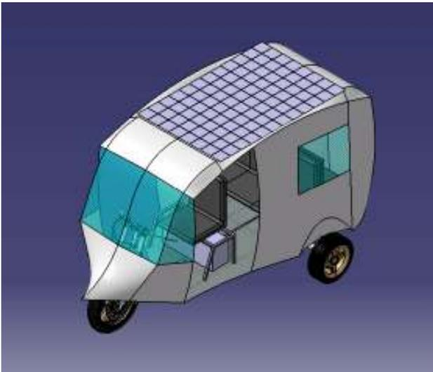
Fig 16. 3D CAD model of the tricycle
