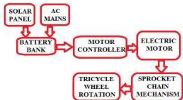
Fig. 8 Block diagram of the electrical system design
