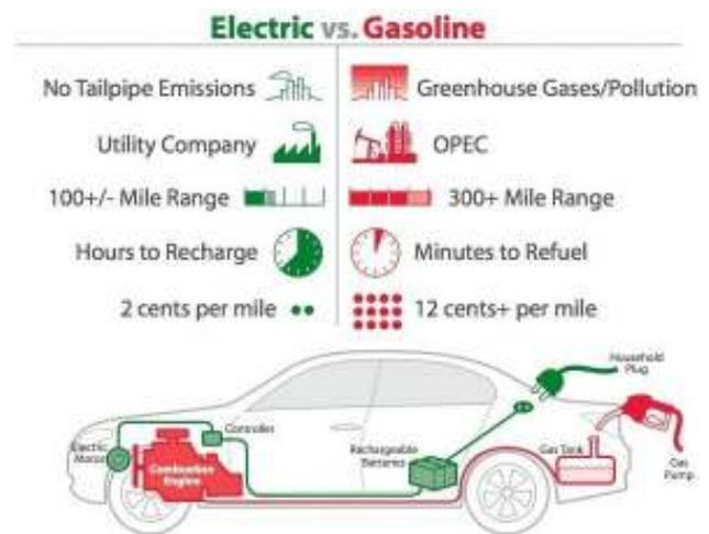
Fig. 1 Electric vehicles against gasoline vehicles [3]
