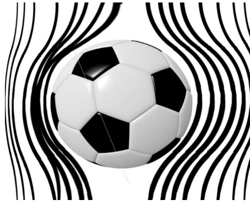
Fig. 6 The difference of pressure that occurs when a gyroscopic momentum is applied on a football.
