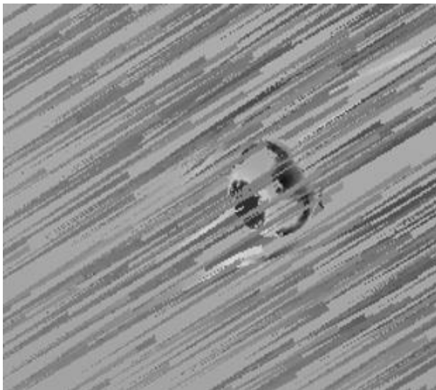
Fig. 11 the behavior of a 439-dimple ball at 60m/s
