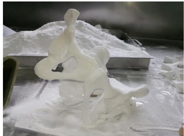
Fig. 8 3D printed hip joint extracted from C.T. scans (made of polymeric material)
