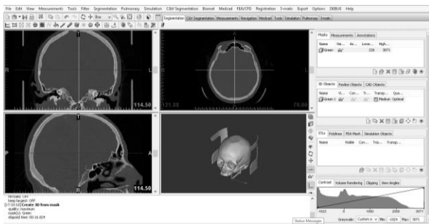
Fig. 4 The .stl surface obtained after the transformation of tomographic images into the Mimics program.
