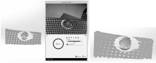
Fig. 9 Inside scan of cup with fixing pins.
