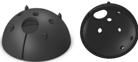
Fig. 10 The three-dimensional parameterized model of the cup with fixing pins.
