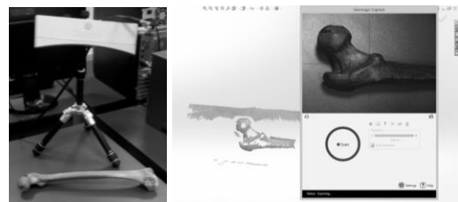
Fig. 1 3D scanner used for a femur taken from a corpse.
