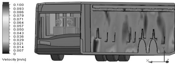
Fig. 9 Velocity of the air distribution.
