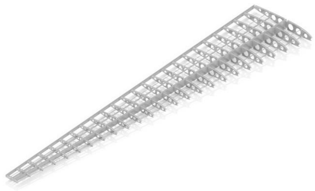
Figure 9 Design of the wing structure
