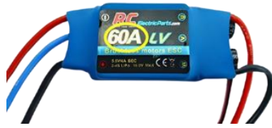
Figure 5. Identifying the rated current on the speed controller [7]
