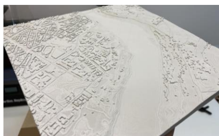
Figure 11 Final model with the 0.2mm layer thickness
