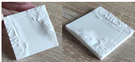
Figure 10 Printing results with the 0.06mm layer thickness
