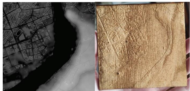
Figure 3 Left – Digital model depth map; Right – Physical model after engraving
