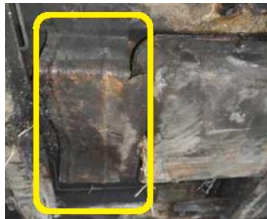
Figure 2 Underbody deformed high voltage cable shield [5].
