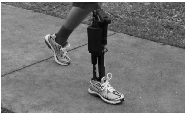
Fig. 3. Walking leg prosthesis for everyday use [13].
