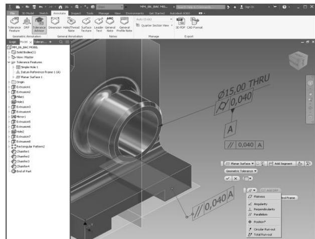
Fig. 6 Adding a position deviation to base "A"
