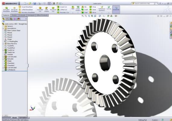
Fig.4. 3D model of bevel gear.
