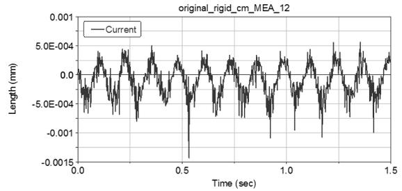
**Fig.18.** Deformation of the shaft center, along the x-axis.
