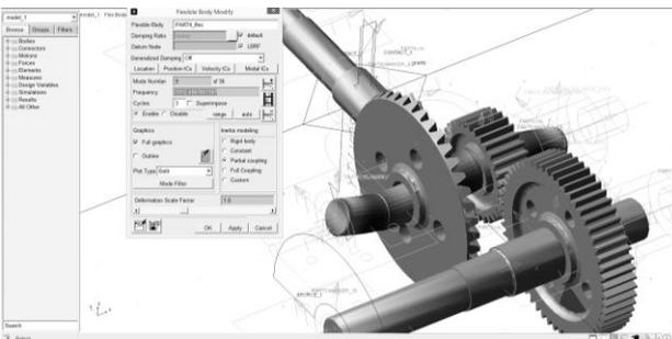
Fig. 23. Deformed representation of shaft II for vibration mode 9.
