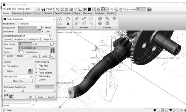
Fig. 30. Deformed representation of shaft I for vibration mode 14.
