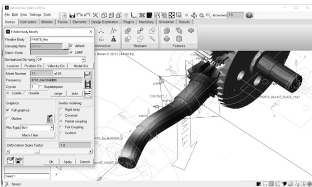
Fig. 29. Deformed representation of shaft I for vibration mode 11.
