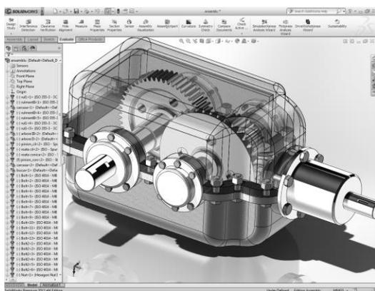
Fig.7. Details of the gearbox CAD assembly.
