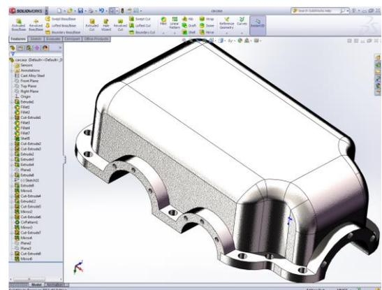
Fig.9. Detail of the gear housing.
