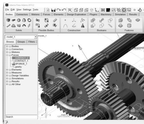
Fig.10. ADAMS dynamic model of bevel-cylindrical gear.
