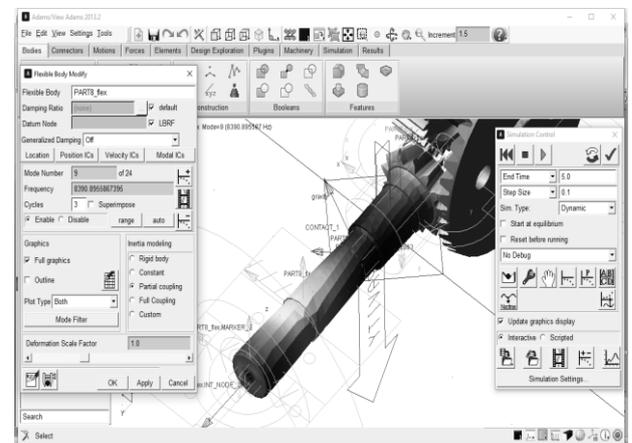
Fig. 27. Deformed representation of shaft I for vibration mode 9.
