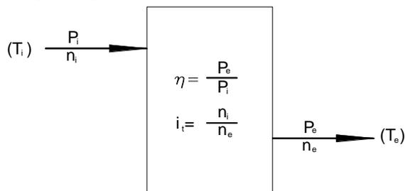
Fig. 1. The kinematic and dynamic parameters of a composite mechanical transmission.
