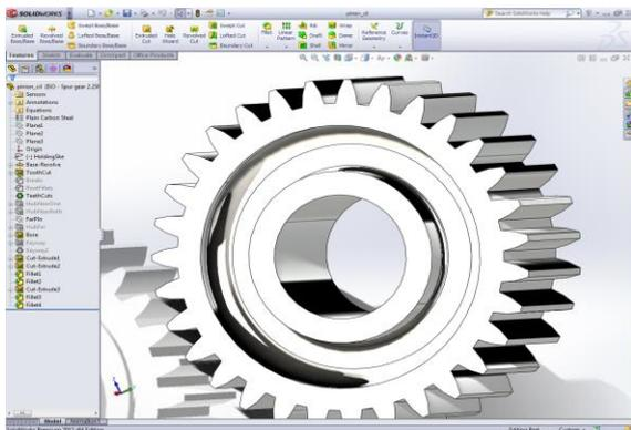
Fig.5. CAD model of cylindrical gear.
