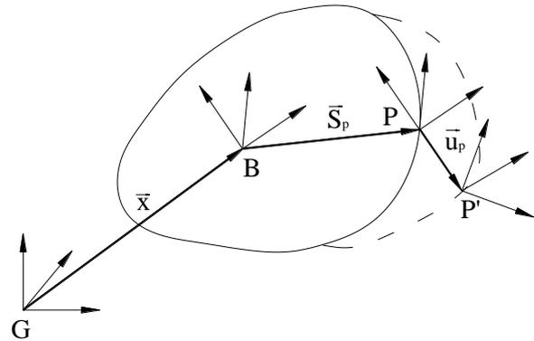
Fig. 13. Deformation point position vector  $P'$  of a flexible body relatively to a reference system attached to body  $B$  and base  $G$ . [8]
