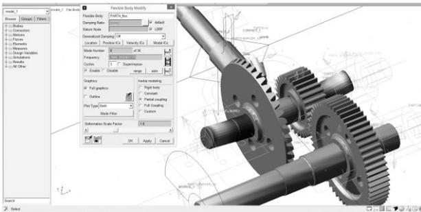
Fig. 22. Deformed representation of shaft II for vibration mode 8.
