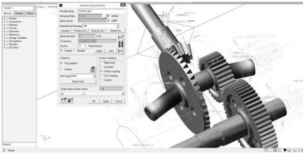
Fig. 21. Deformed representation of shaft II for vibration mode 7.
