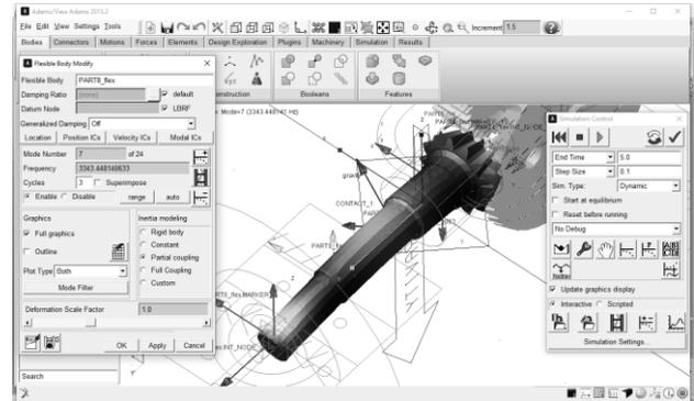
Fig. 25. Deformed representation of shaft I for vibration mode 7.
