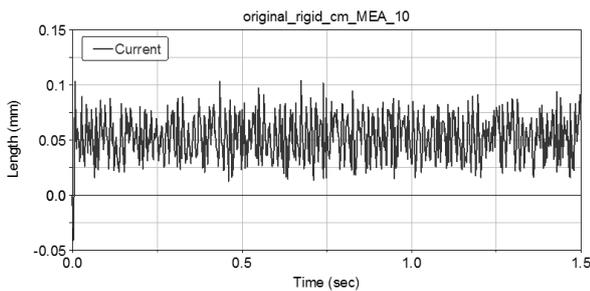
**Fig.17.** Motion of the shaft center, along the z axis.
