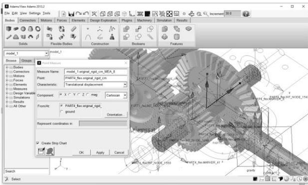
**Fig. 14.** Marker attached to the center of mass of the shaft.
