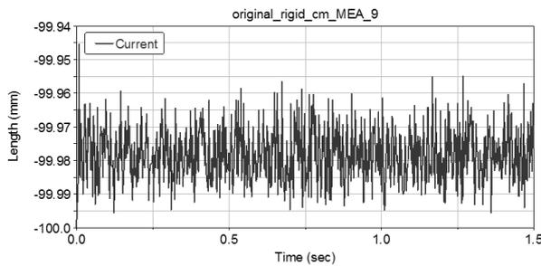
**Fig.16.** Motion of the shaft center on y-axis.
