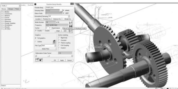
Fig. 24. Deformed representation of shaft II for vibration mode 10.
