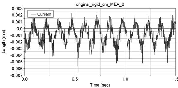
**Fig.15.** Motion of the shaft center, along the x-axis.
