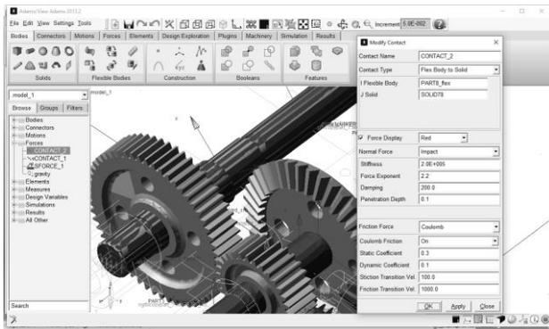
Fig.11. How to define the wheel teeth contact.
