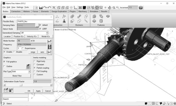
Fig. 28. Deformed representation of shaft I for vibration mode 10.
