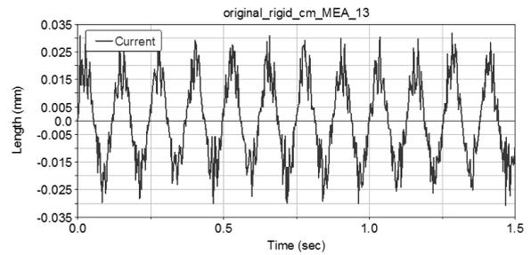
**Fig.19.** Deformation of the shaft center, along the y-axis.
