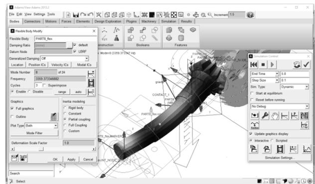
Fig. 26. Deformed representation of shaft I for vibration mode 8.
