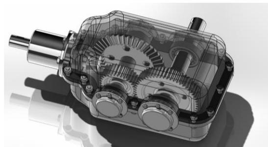
Fig.2. The assembled CAD model of the gearbox.
