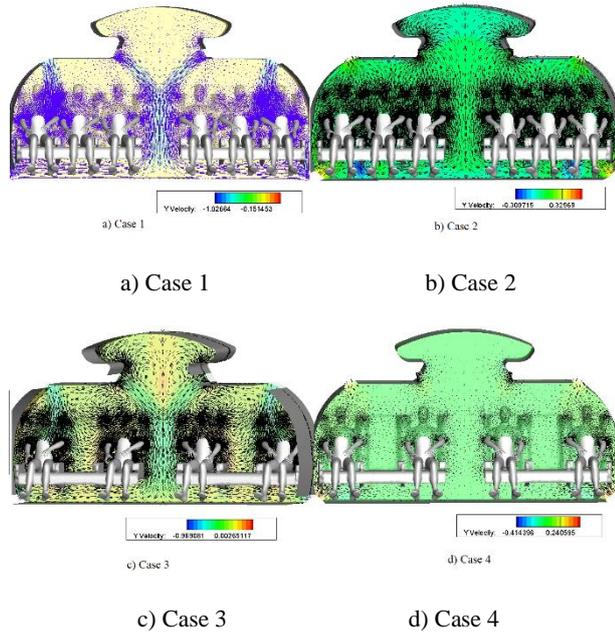
Figure 6 Velocity field in the reference cross-section.
