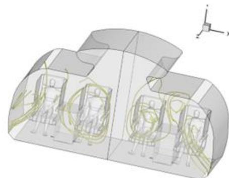
Figure 11 Streamlines in aircraft cabin.
