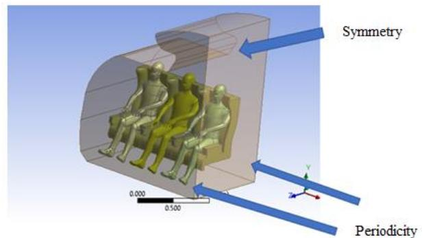
Figure 1 Simplified model with one row of seats and boundary conditions.
