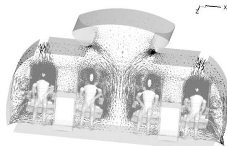
Figure 10 Velocity distribution in the reference section
