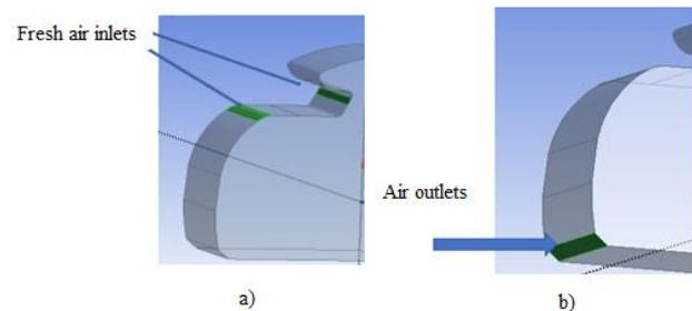
Figure 2 Air inlets and outlets surfaces in mixing ventilation.
