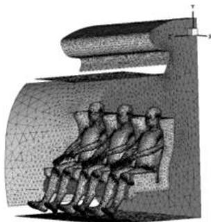
Figure 4 Detail of computational mesh.
