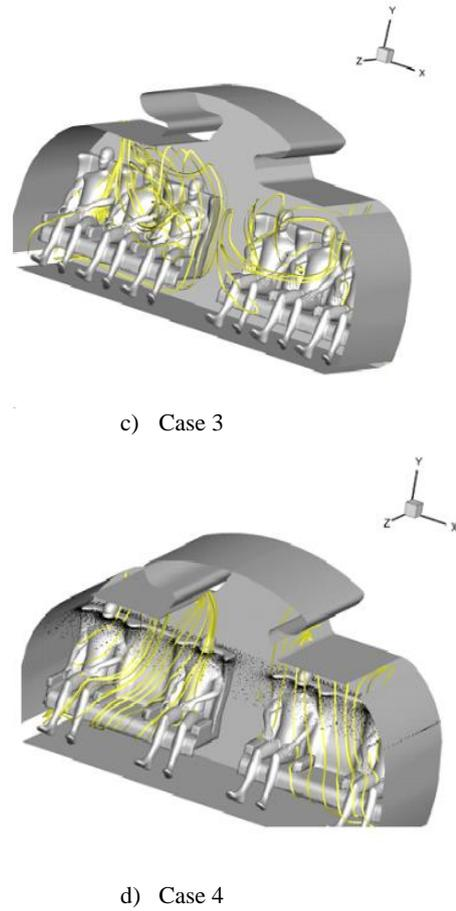
Figure 7 Streamlines in passenger cabin.
