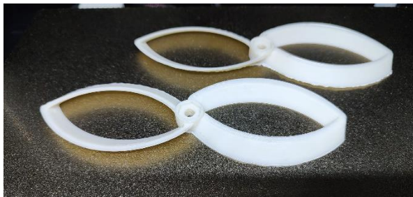
Figure 15 Toroidal 3D printed propeller.
