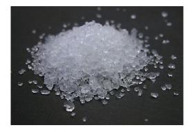
Figure 2 Silica gel pellets.
