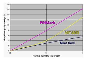
Figure 4 Adsorption capacity in the humidity range 40-60%.
