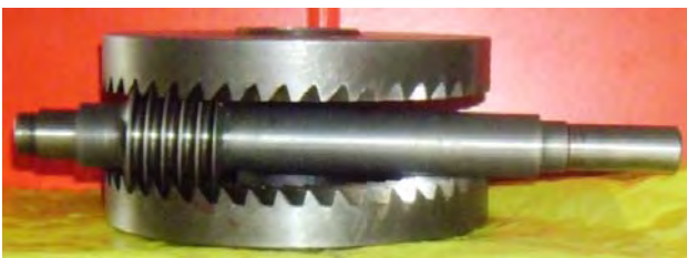
Fig. 1. Double worm-face gear with cylindrical worm
