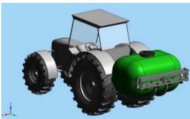
a). Sprayer installation mounted at tractor in the transport position
