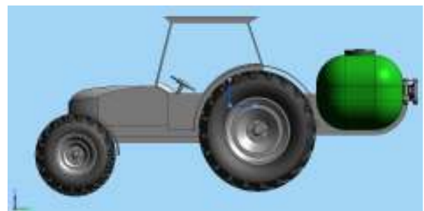
Fig. 2. Assembly of agricultural tractor with sprayer installation attached [9]
