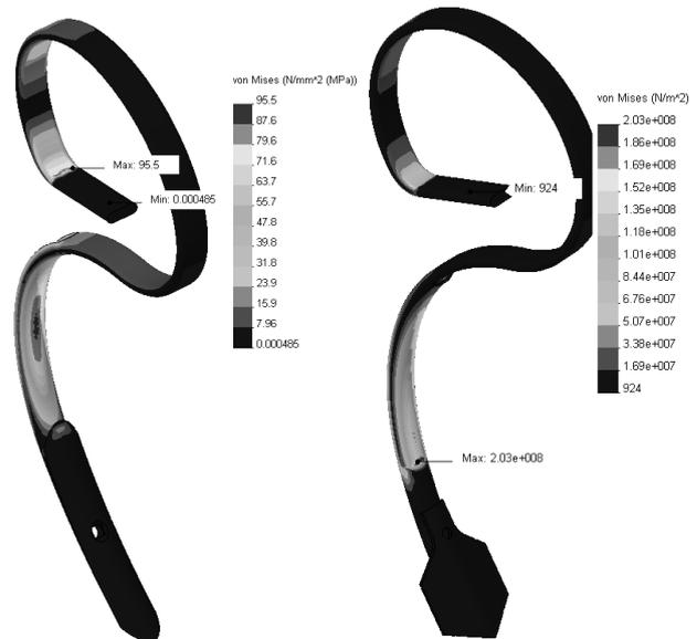
Fig. 11 The tensions of vonMises from the two variants.
