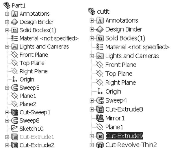
Fig. 3 The CSG tree of the holder and the knife.
