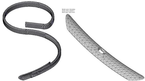
Fig. 7 Meshing of knife and knife support – assembly.
