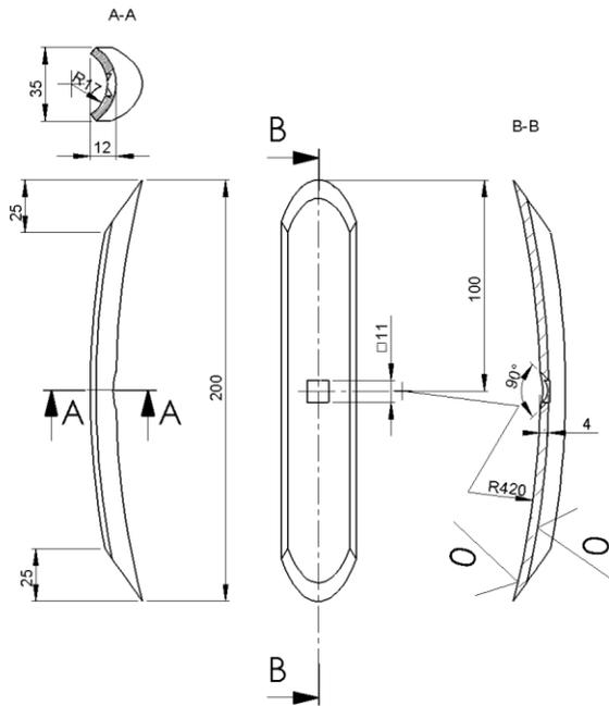
Fig. 5 Chisel shape knife.
