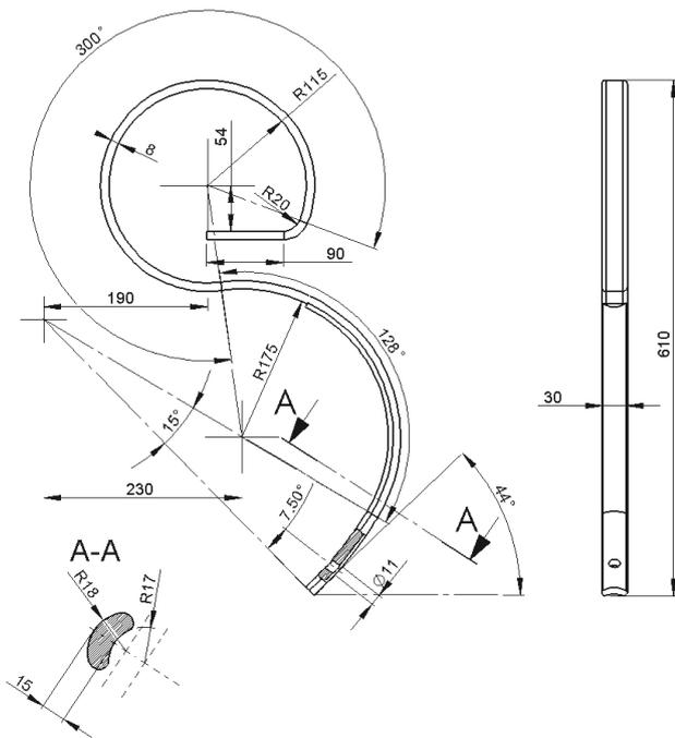
Fig. 6 The dimensioned drawing of the 44° holder.
