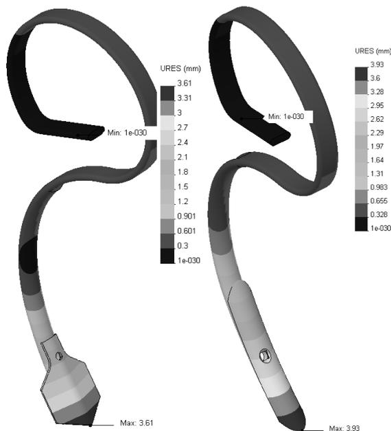
Fig. 12 The nodal displacements in both cases.
