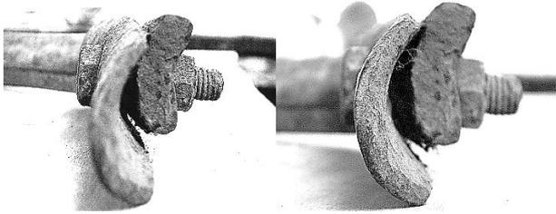
Fig. 9 Bad knife - holder contact/positioning.
