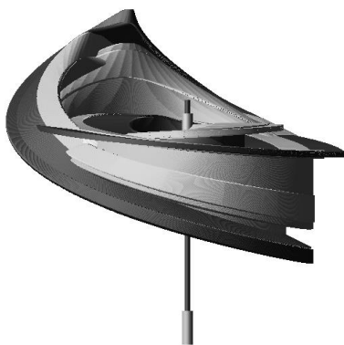
Fig. 6 The kinematic scheme in successive positions, with the RTR generator mechanism.
