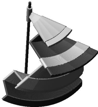
Fig. 20 The sequence in the workspace for the TRRTR mechanism in successive positions.
