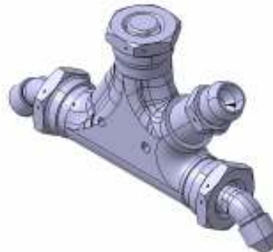
Fig. 7 Mirror symmetry structure of a hydraulic distributor [2]
