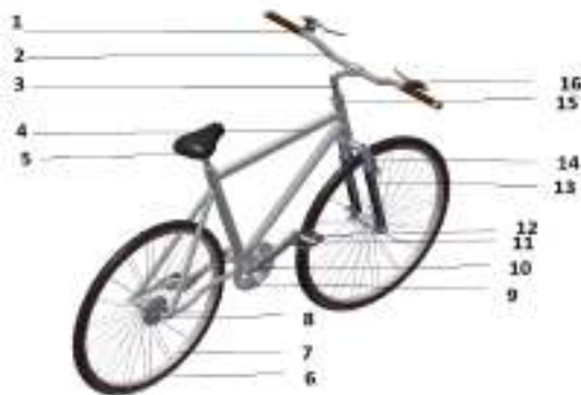
Fig. 4 Parts of the bicycle [9]: 1-handlebar pads; 2-handlebar; 3-fastening clamp; 4-frame; 5-saddle; 6-tyre; 7-rim; 8-wheel sprockets; 9-chainrings; 10-block crank and sheets; 11-crank arm; 12-pedal; 13-suspension fork; 14-upper fork; 15-set bearings; 16-brake.
