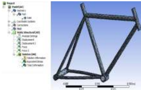
Fig. 15 Hard Tail (HT) frame meshing in ANSYS Workbench using the function Design Modeler.
