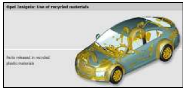
Fig. 4 Using recycled materials represent an important objective in automotive design-for-recycling. [9]
