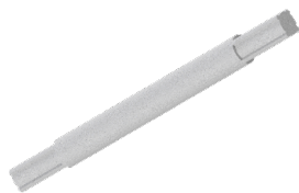
Fig. 7 Radial shaft with grooves.
