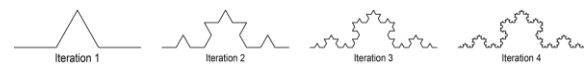
Fig. 3 The first four iteration steps of the Koch curve, a well-known fractal.
