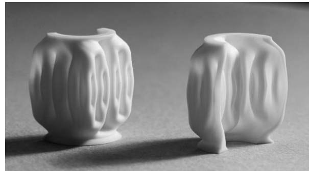
Fig. 10 Another way of designing a transfer surface for a heat exchanger with a FASS curve, here the Hilbert curve. The models show a 5/8 cutout.
